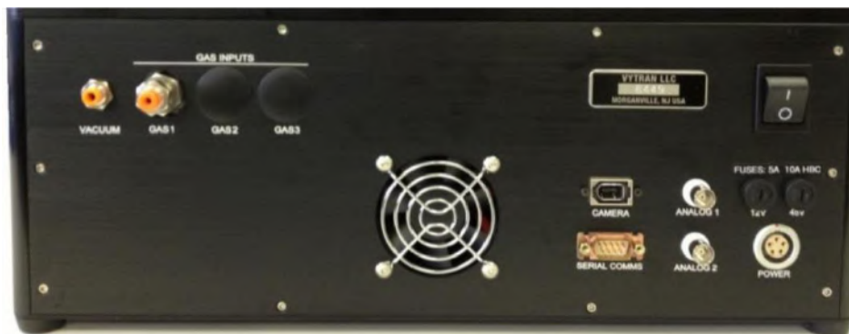
Figure 2 GPX3800 Back Panel Connections
