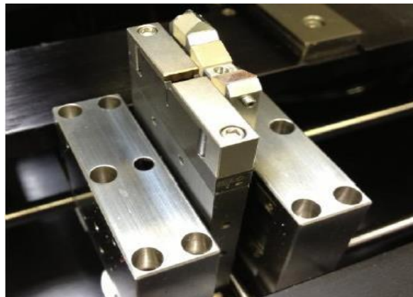
Figure 53 Secure the stainless steel cover plates on the filament assembly
