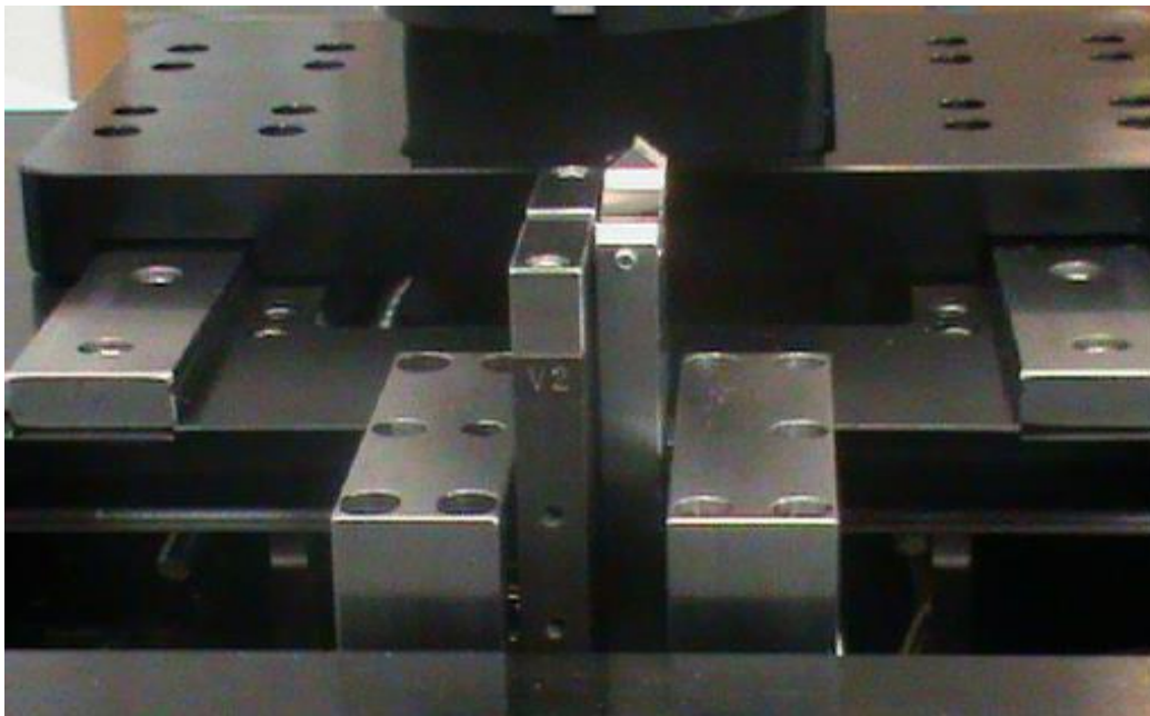
Figure 5 Filament Splice Head
