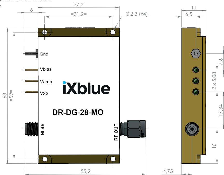
**⚠** The heatsinking of the module is necessary. It's user responsibility to use an adequate heatsink. Refer to page 6 for iXBlue recommended heatsink.
