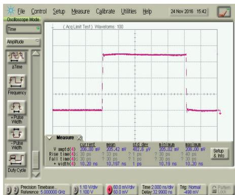
Input signal: Pulse amplitude = 0.24 mV<sub>pp</sub>, Rise time = 32 ps
