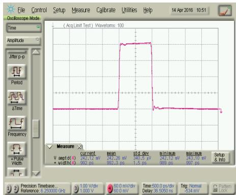
Input signal: Pulse amplitude = 0.242 mV<sub>pp</sub>, Rise time = 32 ps
