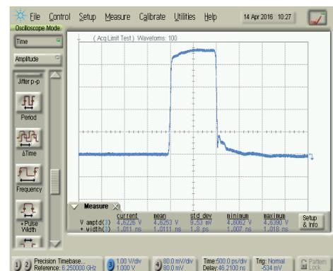
Output response: Pulse amplitude = 4.6 V<sub>pp</sub>, Rise time = 32 ps
