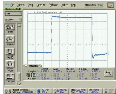
Output response: Pulse amplitude = 4.96 V<sub>pp</sub>, Rise time = 32 ps
