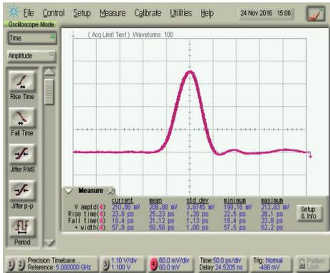
Input signal: Pulse amplitude = 0.227 V<sub>pp</sub>, Rise time = 24 ps
